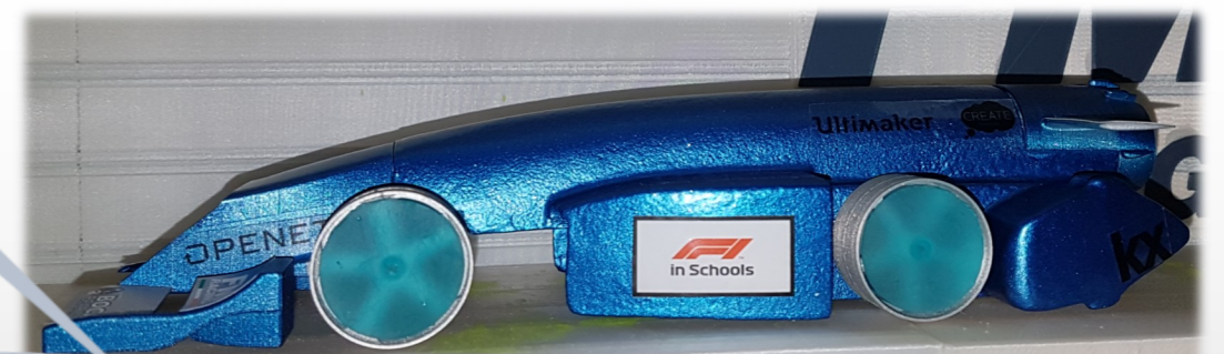
Finished nose cone along with the front wheel bogie, which fits to the rear of the nose. This part features slots inside an aerofoil on each side, which allow the SLA printed axels to fit inside.
