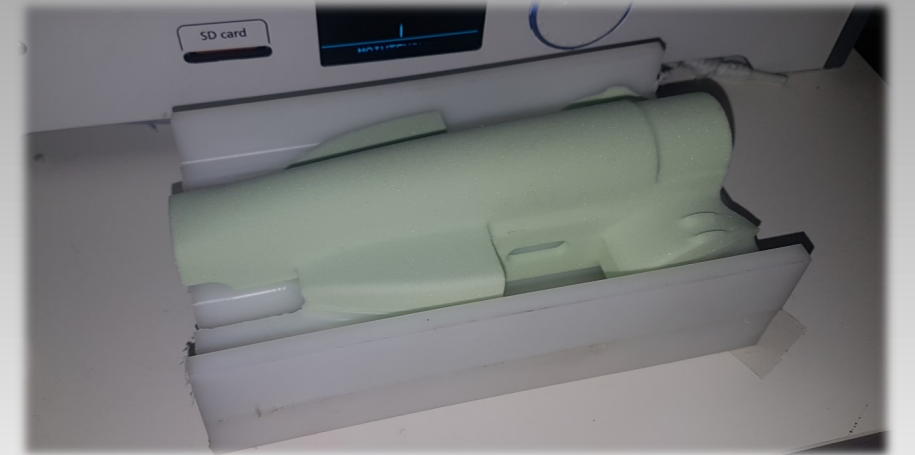
Car body locked in sacrificial plate after completion of manufacturing
