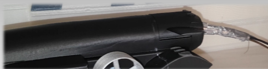
Earlier Vortex generator variant tested in the wind tunnel
