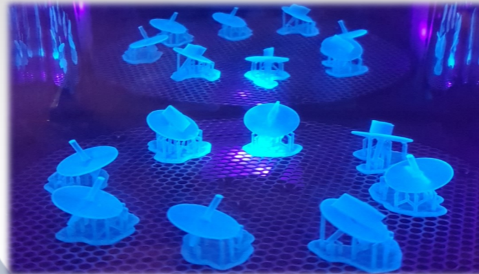
SLA-printed axels with support material during post-curing process
